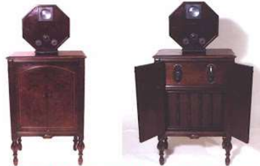
1928 G.E. Scanning Disk Television Set (closed-open)
